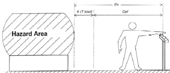
Safety Distance ( $D_s$ ) for a Single Control Device includes a large  $D_{pf}$  of 2 meters (6.5 feet) due to the ability of the operator to stand between the device and reach towards the hazard.
